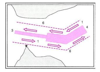
Figure 2 – Traffic separation by separation zone.
