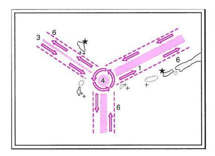
Figure 11 – Separation of traffic at a roundabout
